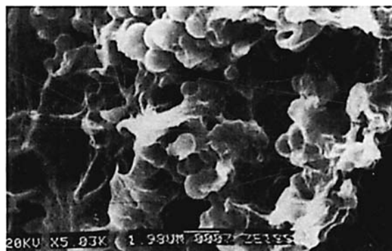
Figure 6 Grain structure of 4000 LL at 5000 \times .
